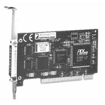
The SyncPCI is sold by Serengeti Systems to provide a synchronous communications port for use with both BSC (byte-synchronous) and SDLC (bit-synchronous) emulation software products. The SyncPCI is also employed in asynchronous mode by these same products to support popular, low-cost auto-dial and auto-answer Hayes compatible 'AT' command set modems.
