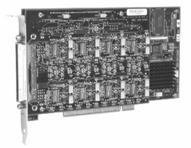
The SmartSync/DCP is sold by Serengeti Systems to provide up to eight synchronous communications ports for use with BSC (byte-synchronous) emulation software products. The SmartSync/DCP is also employed in asynchronous mode by these same products to support popular, low-cost auto-dial and auto-answer Hayes compatible 'AT' command set modems.
