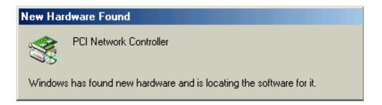
The Windows **Add New Hardware Wizard** is used to install the necessary driver software as shown below (example from Windows Me -- the dialog box you actually see may be different):
