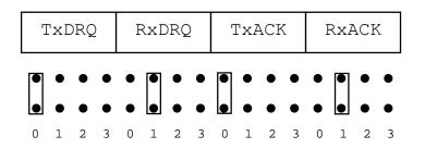
It does not matter which DMA channel you use for transmit or receive as long as they are not the same and are otherwise unused by your PC.
