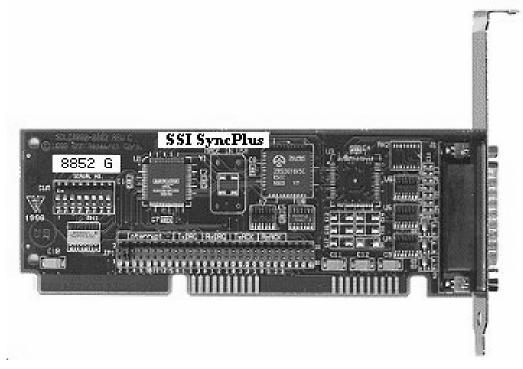
The SyncPlus is sold by Serengeti Systems to provide a synchronous communications port for use with both BSC (byte-synchronous) and SDLC (bit-synchronous) emulation software products. The SyncPlus is also employed in asynchronous mode by these same products to support popular, low-cost auto-dial and auto-answer Hayes compatible modems.
