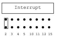
On some PC's with a Plug-n-Play (PnP) BIOS, special attention is required when you install any ISA-bus adapter that is not PnP aware – the SyncPlus falls into this category. Often it is necessary to reserve the IRQ (and DMA channels) used by a non-PnP adapter in the BIOS configuration at boot time. If this applies to you, consult with your system administrator or the PC's documentation about how to reserve an IRQ for use with the SyncPlus (more on this later in this setup guide).
